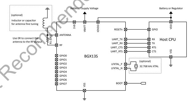
Figure 3.1. Typical Connections for BGX13S
