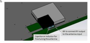
Figure 4.3. Practical Installation of BGX13S on Application PCB
