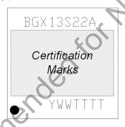
Figure 7.4. BGX13S Package Marking
