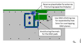
Figure 4.1. BGX13S PCB Top Layer Design
