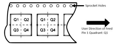
Figure 8.4. Module Orientation and Feed Direction
