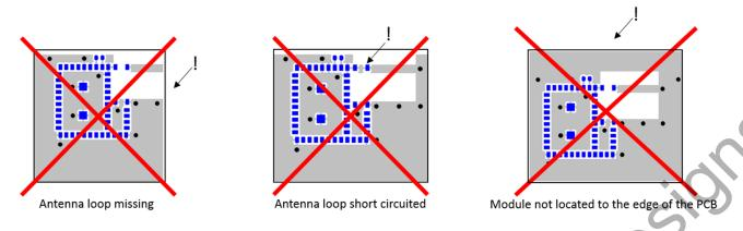
Figure 4.4. Poor Layout Designs for the BGX13S
